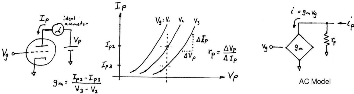
**Figure 1.** Transconductance Definition and AC Tube Model
