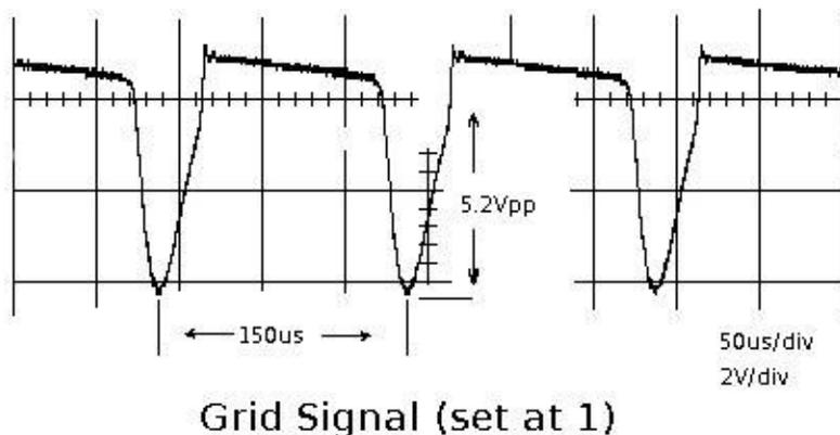
**Figure 3.** TT-1 Transconductance Test Grid Signal
