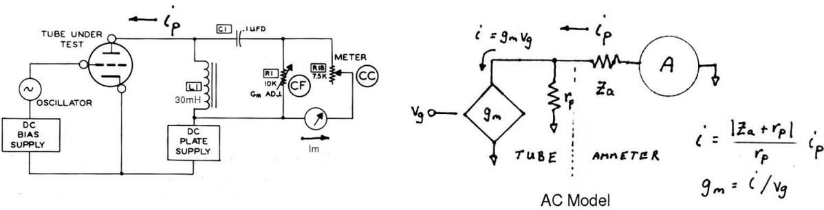
**Figure 2.** TT-1 Measurement Configuration and AC Model
